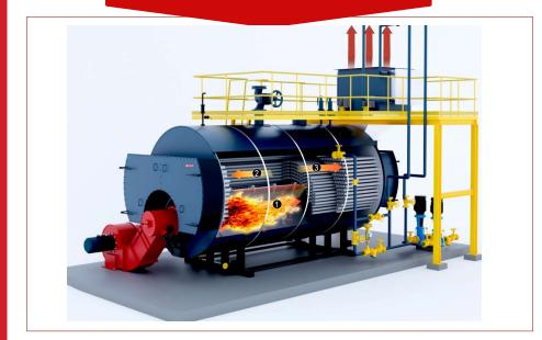
3D internal flue gas flow for 4-pass
